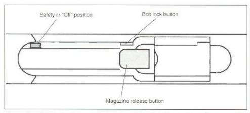
The underside of the trigger guard section in the rifle. In this illustration the safety is shown in the "OFF" (FIRE) position. The red band indicates the safety is "OFF"
