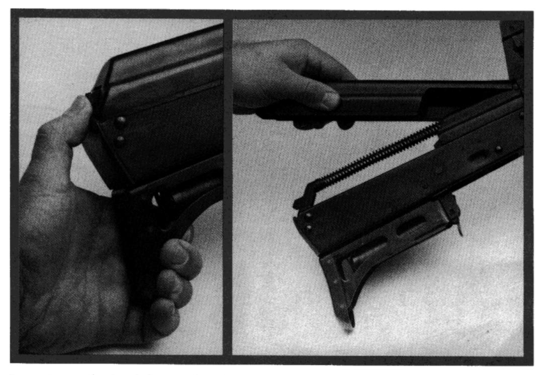
Press in on the latch located at the top rear of the rifle and lift the top cover off.
