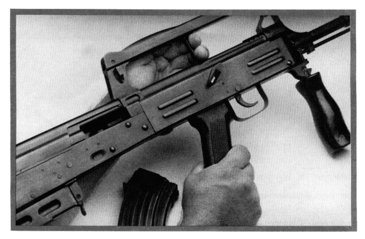
**DISASSEMBLY:** To disassemble the 86S for cleaning and maintenance, first remove the magazine and pull the bolt back to check and see that the chamber is empty and no ammunition is in the rifle.
