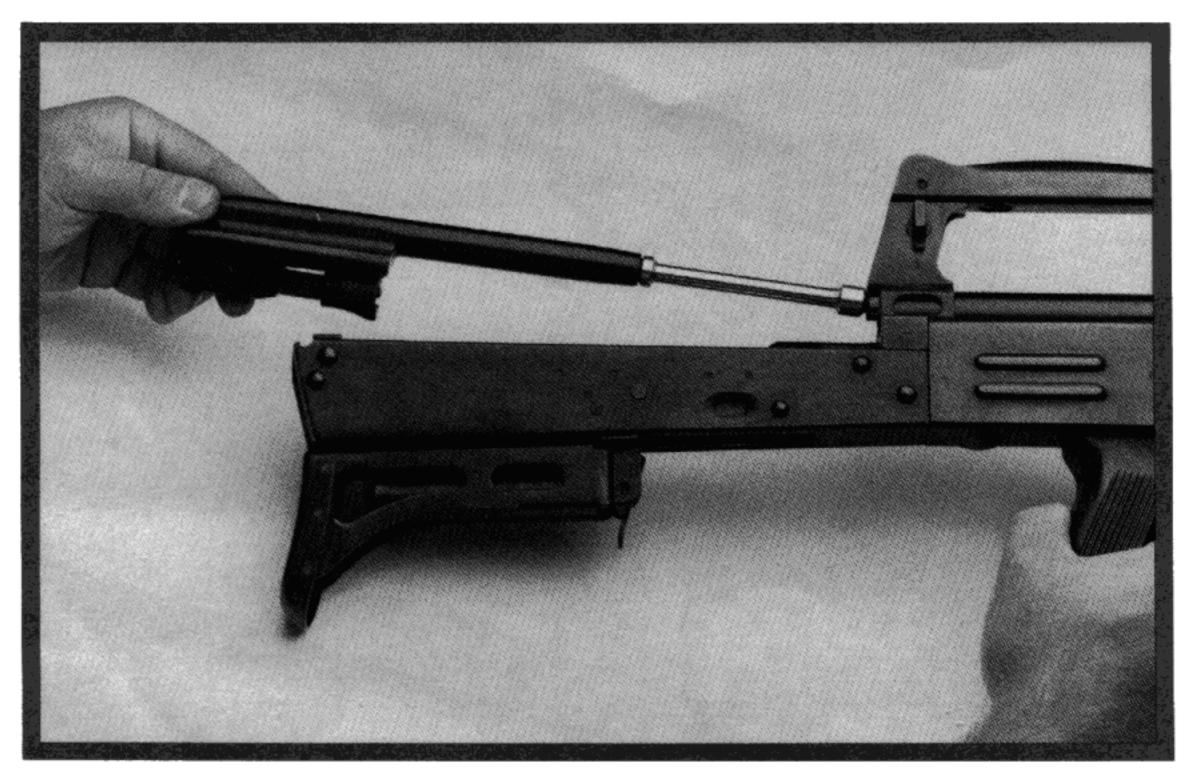
The bolt and bolt carrier are now free to be removed from the rifle.
