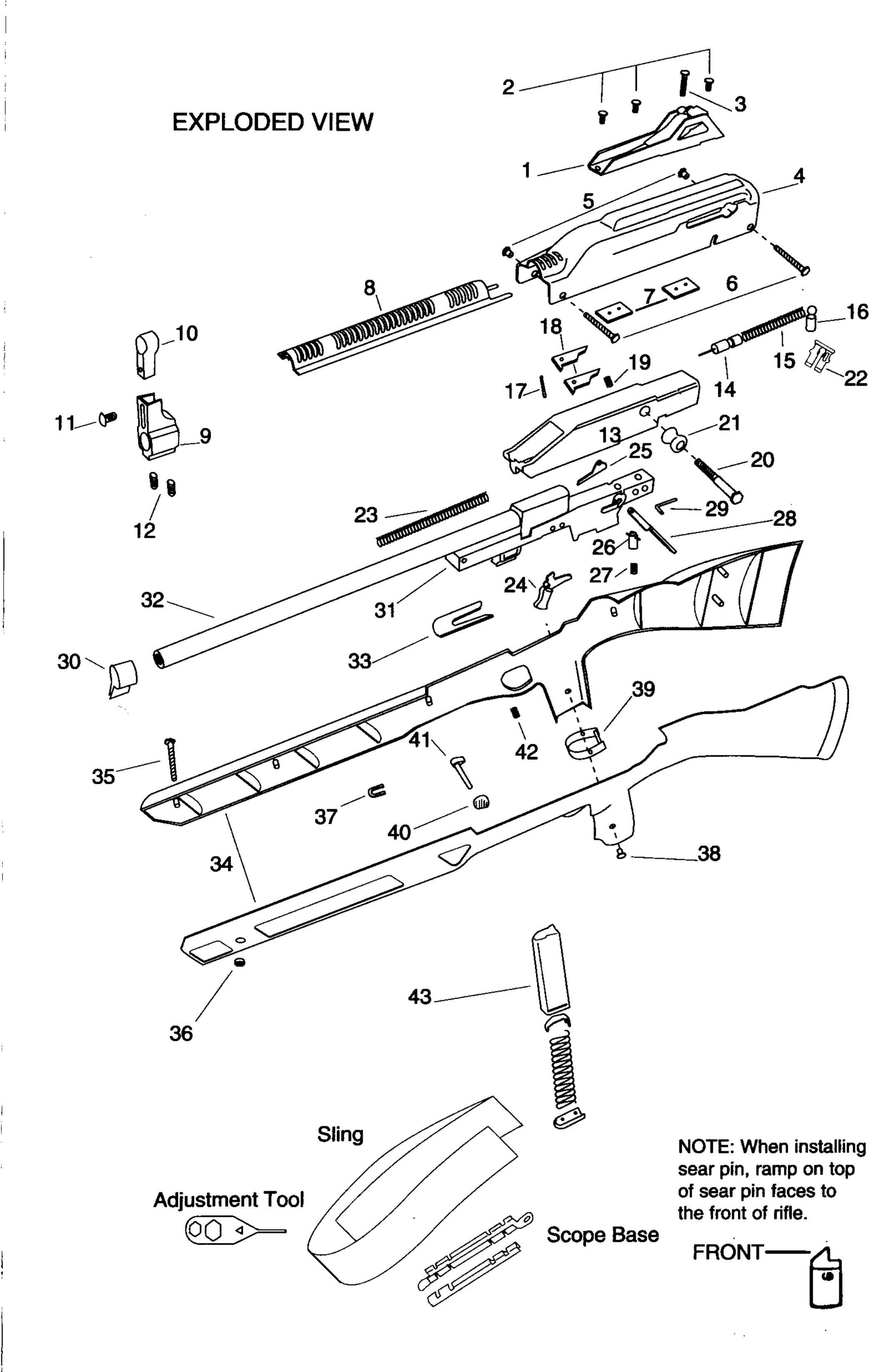
Safety/Bolt Lock is located at top of left grip. Sliding safety lever upward, into notch engages safety and places rifle in "SAFE" position.
